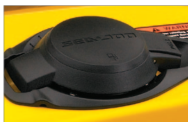
Quick latch fuel filler design
