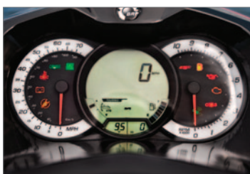
Digital information centre with speedometer
