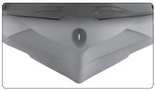
**T3-R<sup>™</sup> Hull** A deep-V design that offers unrivaled handling and acceleration and a new level of control at high speed.
