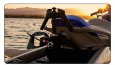
LinQ Retractable Ski Pylon A quick-install retractable ski pylon that stows away when not in use. Features spotter handgrips and rope storage.
