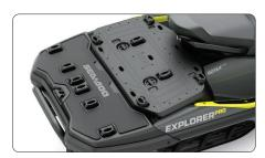
Rear Deck Extension with LinQ Attachment System and Multi Cargo Rack
