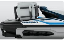
Extended Rear Platform with Second LinQ<sup>®</sup> Attachment System Adds 11.5 inches to the back of the watercraft to increase stability, space, and storage capability.
